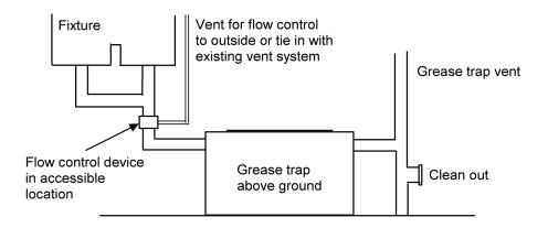
Typical multiple fixture grease trap installation
