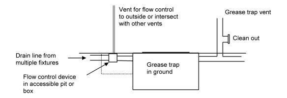
Typical Indirect fixture grease trap installation
