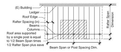
Loading: DL = 10 psf. (Roofing Material = 6 psf max.) LL = 10 psf.
