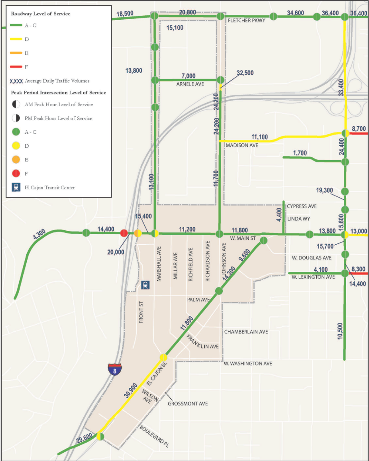
Figure 3 Existing Roadway Average Daily Traffic Volumes & Level of Service and Intersection Level of Service
